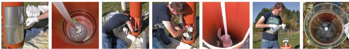
sample collection and funnel flushing
