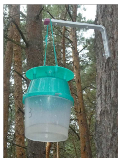
Fig. 1: VarioTrap® pheromone trap for monitoring forest pest Lepidopterans. (R. Fritz)
